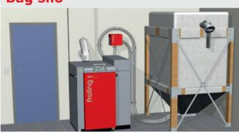
The bag silo system is a flexible, simple way of storing pellets. Available in 9 different footprints (from 1.5 m x 1.25 m to 2.9 m x 2.9 m) with a capacity of between 1.6 and 7.4 tonnes, depending on the bulk density.
